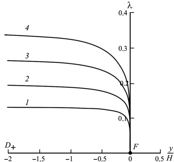
**Fig. 3.** The distribution of the amplitude of the pressure coefficient on the wall  $D_+F$  for  $\omega = 1, 2, 3, 4$  (curves 1–4, respectively) and for  $\varepsilon = 0.1, q_0 = 0.7$ , and  $Z_C = -0.54H + 0.5Hi$ .
