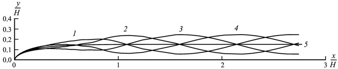
**Fig. 2.** The shape of the free boundary *FB* for  $\tau = 3\pi/4, 0, \pi/4, \pi/2$  (curves 1–4, respectively) and for  $\omega = 1, \varepsilon = 0.1, q_0 = 0.7$ , and  $Z_C = -0.54H + 0.5Hi$ ; (5) the stationary free surface.
