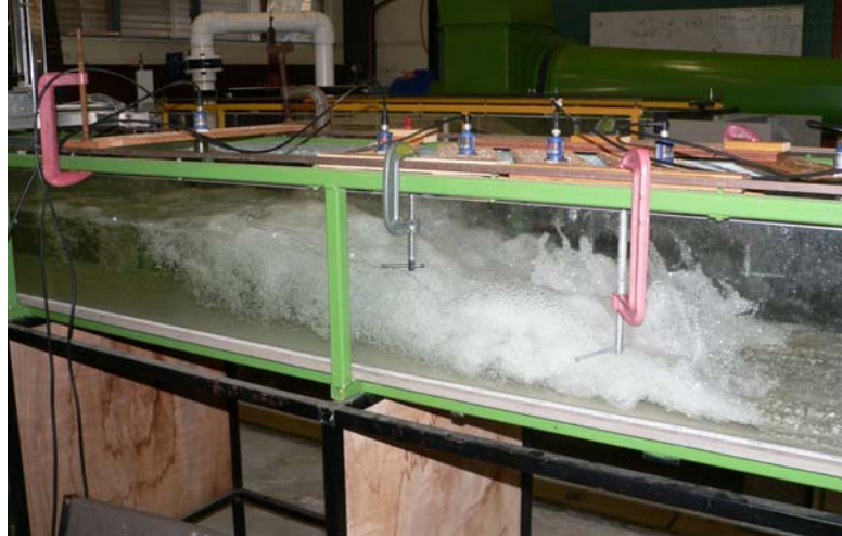
(B) Hydraulic jump with roller: Fr_1 = 7.9 , d_1 = 0.018 m, Re = 5.9 \cdot 10^4 , B = 0.5 m- Flow from right to left
