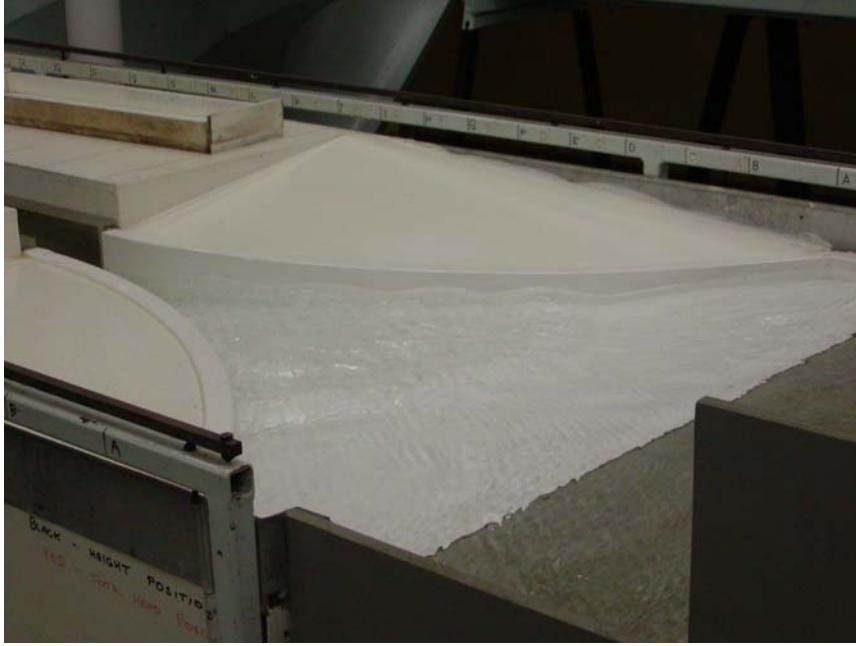
(A) Photograph of the smooth drop inlet experiment - Flow from bottom right to top left
