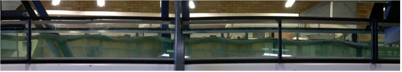
(A) Undular hydraulic jump: Fr_1 = 1.1 , d_1 = 0.104 m, Re = 1.1 \cdot 10^5 , B = 0.5 m- Flow from right to left
