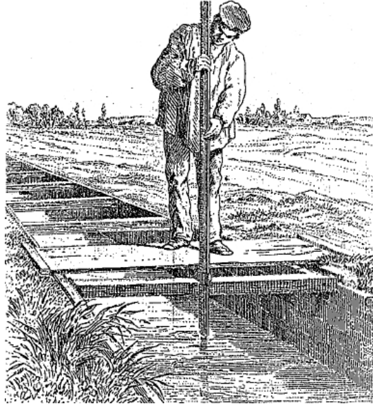
(C) Free-surface measurement (DARCY and BAZIN 1865, Plate iv, Fig. 8)
