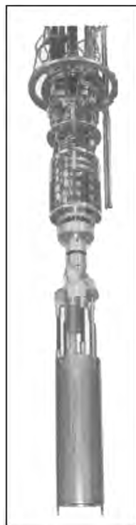
Fig. 6.8. Miscibility gap in \text{He}^3 - \text{He}^4 phase diagram (schematic). Enriching \text{He}^3 in the \text{He}^3 -rich phase by evaporation. \text{He}^3 - \text{He}^4 cryostat of the Physikalisch Technische Bundesanstalt in Berlin. 33
